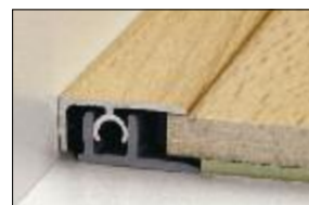
Profitec end profile Two-part aluminium profile, e.g. for transitions between floors and walls. For floor thicknesses of 8–14 mm. 28 mm × 1 m | 2,7 m
