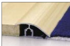
Profitec adaptation profile Two-part aluminium profile for transitions between floors of varying heights. For floor thicknesses of 7–17,5 mm. 47 mm × 1 m | 2,7 m
