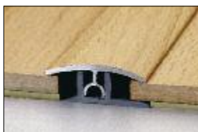
Profitec transition profile Two-part aluminium profile for covering expansion joints. For floor thicknesses of 7–15 mm. 34 mm × 1 m | 2,7 m
