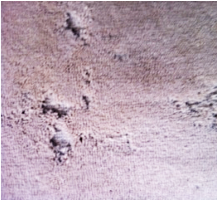
Signs of moth damage to a fitted carpet
