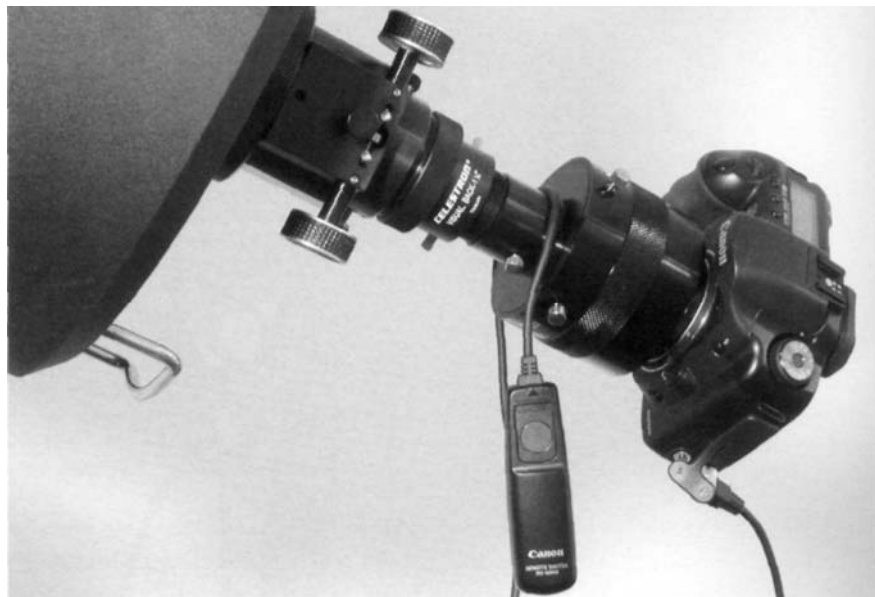
Fig. 5.14 The Scopetronix MaxView DSLR Variable Projection Adapter can be used as a prime focus coupler by removing the eyepiece and collapsing the projection body. Photo by Robert Reeves.
