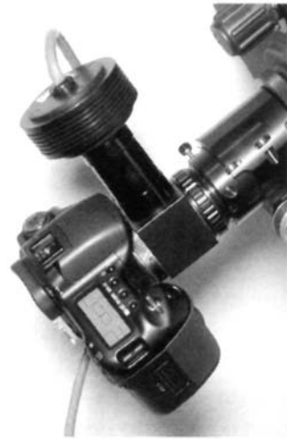
Fig. 9.7 The development of electronic autoguiders such as the Santa Barbara Instrument Group ST-4 has allowed the astrophotographer to achieve flawless long exposures without fatiguing and tedious manual guiding. Photo by Robert Reeves.
