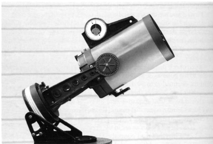
Fig. 9.2 A rough polar alignment can be done in the daytime by using an inclinometer to adjust the polar axis elevation and a compass to point the polar axis toward north. Photo by Robert Reeves.
