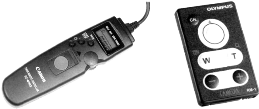
Fig. 8.10 Left) Electronic cameras need electronic remote shutter releases. The Canon TC80-N3 for the EOS 10D is typical and is also capable of controlling a sequence of preprogrammed time exposures. Photo by Robert Reeves. (Right) Many compact digital cameras are capable of remote shutter operation using a wireless infrared remote switch. The Olympus Camedia series uses the RM-1 wireless remote shown above. Photo courtesy of Olympus.
