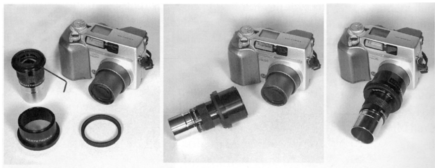
Fig. 8.2 The Scopetronix Digi-T system will adapt compact digital cameras to most 1\frac{1}{4} -inch eyepieces that have a removable rubber eyeguard. The Digi-T-adapter is attached to the machined rim of the eyepiece with three setscrews (left). A step ring and lens adapter collar is then threaded onto the Digi-T-adapter (center), and the entire eyepiece and adapter assembly then threads into the camera lens or camera body (right). Photos by Robert Reeves.
