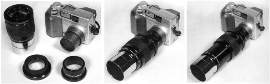
Fig. 8.7 The MaxView II 40-mm 2-inch eyepiece allows compact digital cameras to be coupled to 2-inch focusers and achieve a wider field-of-view than available with the standard 1 \frac{1}{4} -inch MaxView 40. The rubber eyeguard adapter is unthreaded from the top of the eyepiece and a step ring attached in its place (left). The same lens collar used with the Digi-T system is then attached to couple the camera to the eyepiece (center). Photos by Robert Reeves.
