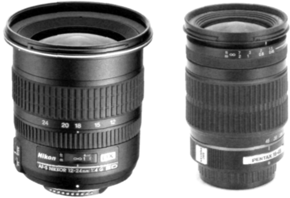
Fig. 7.6 The majority of lenses designed for DSLR cameras are zoom lenses. These "digital-friendly" lenses are longer in physical length than their short focal length would normally indicate because of the digital sensor's need for a lens with a high exit pupil. A disadvantage for astrophotographers is the fact that most digital looms feature a small aperture. Photos courtesy of Nikon and Pentax.
