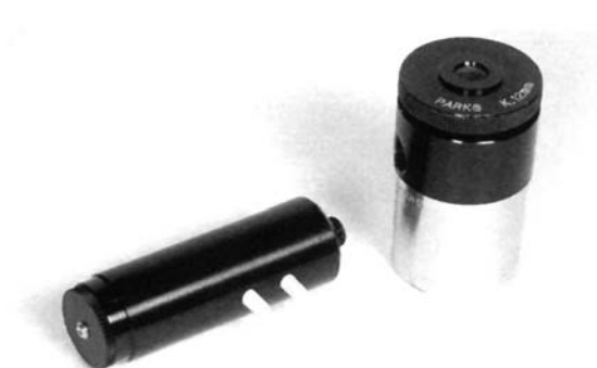
Fig. 9.5 Existing wire-powered illuminated guiding eyepieces can be converted to wireless operation by installing an aftermarket battery and illuminator such as the PulseGuide offered by Rigel Systems. The two knobs adjust brightness, and control adjustable-duration blinking illumination. Photo by Robert Reeves.
