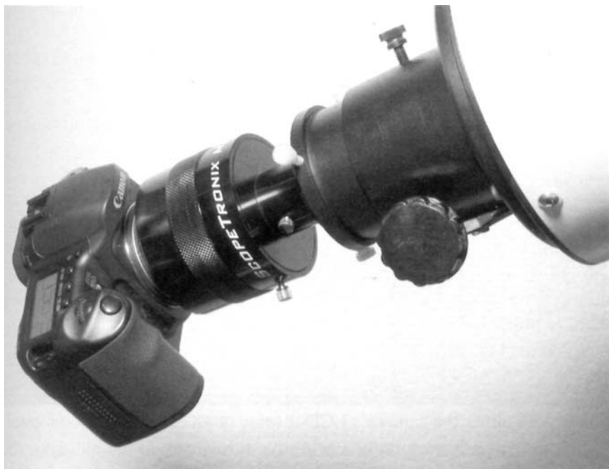
Fig. 5.24 The Scopetronix MaxView DSLR Variable Projection Adapter allows eyepiece projection with DSLR cameras using standard T-adapters. The MaxView is big enough to hold virtually any eyepiece, even the huge 31-mm Nagler or 41-mm Panoptic. The adapter is available in 1.25-inch and 2-inch versions and can be used without an eyepiece as a prime focus adapter. If lack of backfocus limits the usefulness of MaxView, an included telenegative lens can be used to increase the focal length of the system to where focus can be achieved. Photo by Robert Reeves.
