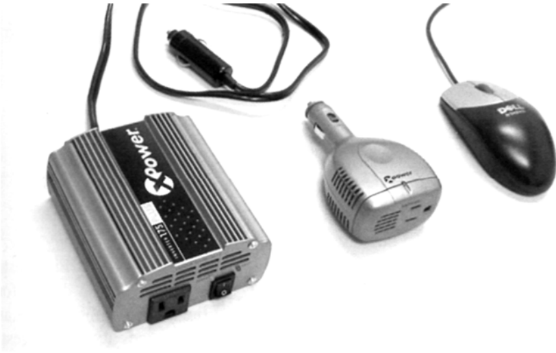
Fig. 8.12 Inexpensive widely available 12-volt inverters manufactured by companies such as Xantrex can power low-wattage accessories such as 120-volt powered battery eliminators for digital cameras. Photo courtesy of Xantrex.
