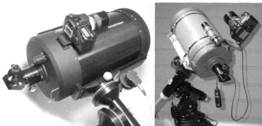
Fig. 5.8 Piggyback astrophotography involves attaching a camera to an equatorially mounted telescope with a suitable adapter. As the telescope follows the stars, it allows the camera to also properly track the stars. (Left) A camera can be mounted on top of the telescope for horizontal "landscape" views or mounted sidesaddle to record vertical "portrait" oriented views. If the telescope is too small to allow convenient sidesaddle mounting, a 90-degree angle bracket can be made from \frac{1}{4} -inch steel to orient the camera for vertical views. (Right) Photos by Robert Reeves.
