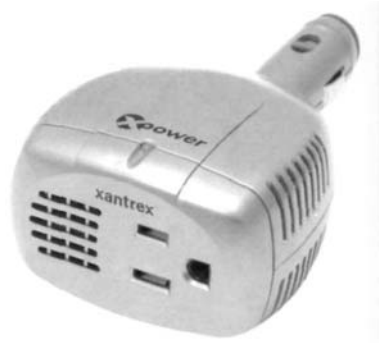
Fig. 8.13 Low-wattage 120-volt accessories can be powered at remote locations using a 12-to-120 volt inverter that plugs into a cigarette-lighter socket. Units such as the one here are manufactured by Xantrex and marketed by popular outlets such as Radio Shack. Photo courtesy of Xantrex.
