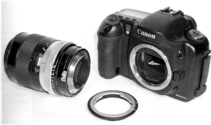
Fig. 7.4 If you already own a number of Nikon film camera lenses but desire to use a Canon DSLR body, Novoflex makes the NIK EOS adapter that will allow the use of Nikkors on an EOS body. Photo by Robert Reeves.
