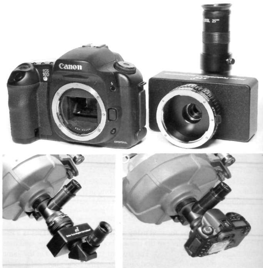
Fig. 11.4 Knife-edge focusers, such as the Stillete IV made by Stellar Technologies International, are substituted for the camera body and use a Ronchi grating to achieve exact telescope focus. The telescope focuser is then locked (lower left), and the camera body installed in place of the knife-edge focuser (lower right). Photos by Robert Reeves.
