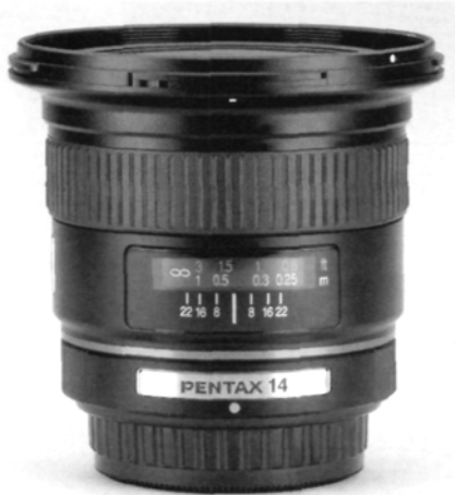
Fig. 7.7 Fixed-focal length "digital-friendly" lenses also retain the trait of being physically longer than their same focal length film camera lenses. This Pentax 14-mm lens is as long as some popular 85-mm lenses used on film cameras. The physical length is dictated in part by the need for greater exit pupil to focal plane distance in order for light rays exiting the lens to be as parallel as possible to properly illuminate the digital imaging sensor. Photo courtesy of Pentax.
