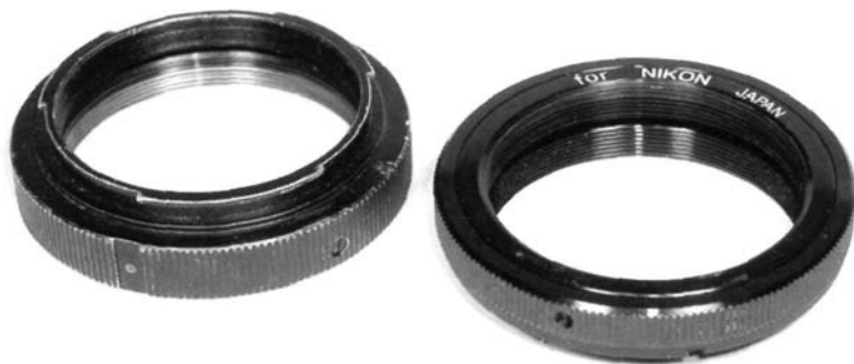
Fig. 5.12 A T-ring, or T-adapter, is used to mount different camera bodies to accessories that use a common mounting thread. The camera side of the T-adapter (left) is specific to the type of camera body used while the threaded accessory side of the adapter (right) uses the same threads for all T-adapters. Photo by Robert Reeves.
