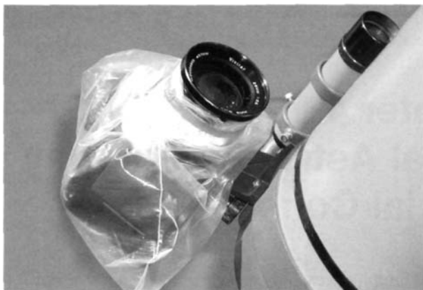
Fig. 4.1 If dew is a problem, camera electronics can be protected by enclosing the camera body in a plastic bag with the lens protruding through the bag opening and sealed with a rubber band. Photo by Robert Reeves.
