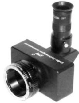
Fig. 5.21 The Stiletto knife-edge focuser marketed by Stellar Technologies takes the guesswork out of focusing on stars by using a Ronchi grating to show a telescope's exact focus point for a given brand of DSLR camera. Photo by Robert Reeves.
