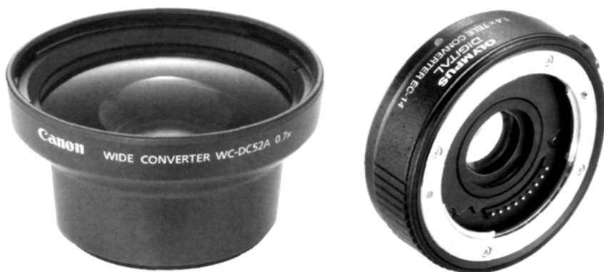
Fig. 7.12 Wide-converters (left), that thread into the front of a camera lens, or teleconverters (right) that fit between the camera body and lens, are popular ways to gain either a wider field-of-view or greater focal length with a given lens. Neither are recommended for astrophotography because they introduce additional aberrations and the image quality suffers. Photos courtesy of Canon and Olympus.
