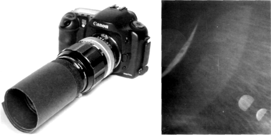
Fig. 8.1 (Left) If the filter being used on a telephoto that has a built-in lens shade is too large to allow the shade to extend, a simple solution is to make a lens shade out of black construction paper and tape it in place. The shade should extend 1.5 times the clear aperture of the lens. (Right) The need for a lens shade, even at night, is illustrated by this image of an Iridium satellite flare. If a lens shade had been used, a nearby light would not have ruined the image by causing reflections and light-scatter within the camera lens elements. Photos by Robert Reeves.
