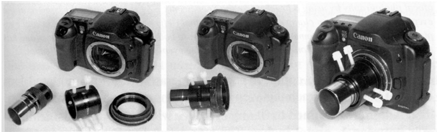
Fig. 8.4 Any camera capable of accepting a T-mount can be coupled to odd-sized eyepieces on binoculars or spotting scopes using the Scopetronix Uni-T-adapter. A standard T-adapter threads onto the Uni-T while the nylon set-screws clamp the unit onto any eyepiece between \frac{1}{4} and \frac{1}{2} -inches in outside diameter. Photos by Robert Reeves.
