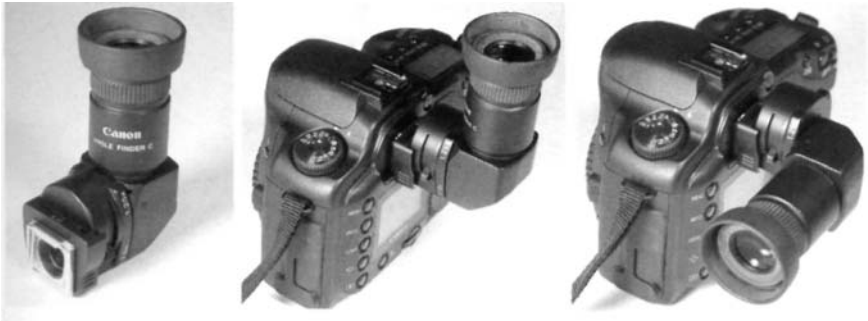
Fig. 4.11 To focus and frame dim targets through the smaller viewfinder in DSLR cameras with less than full-frame image sensors, a magnifying finder, such as the Canon Angle Finder C used on the EOS 10D, is a helpful accessory (left). The finder has variable magnification and can be swiveled for convenient viewing (middle and right). Photos by Robert Reeves.
