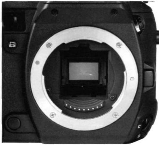
Fig. 4.3 The Olympus E1 is one of the first cameras to actively combat dust on the imaging sensor. An ultrasonic "shaker" dislodges dust on the surface of the sensor every time the shutter is triggered. Photo courtesy of Olympus.
