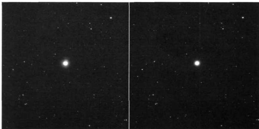
Fig. 11.18 Most lenses render ultraviolet and shorter blue wavelengths slightly out of focus while wavelengths in the middle of the visible spectrum focus well. This causes blue halos around brighter stars (left). A Minus-violet filter will eliminate the far end of the blue spectrum and reduce the blue halos around bright stars (right). Photos by Robert Reeves.
