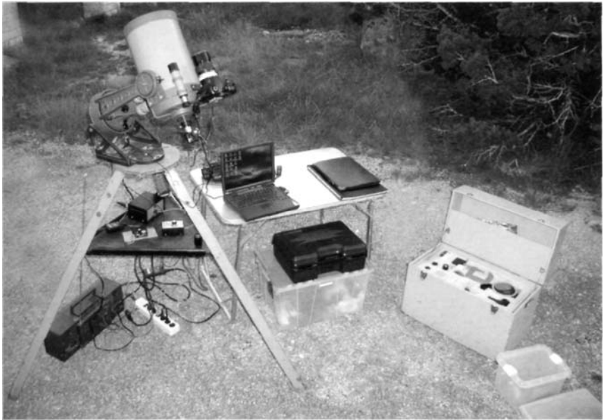
Fig. 5.7 The author's piggyback astrophotography setup is typical of those using a DSLR mounted on a small telescope. A laptop at the telescope is a normal part of digital imaging. Photo by Robert Reeves.
