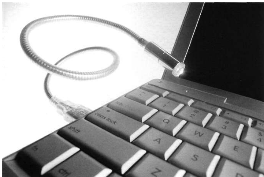
Fig. 11.25 A flexible USB-powered plug-in light can provide low-level continuous keyboard illumination. Photo courtesy of Hoodman.
