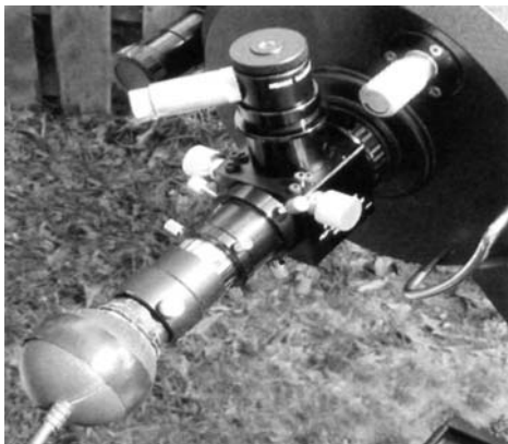
Fig. 2.10 Locating a planet in a webcam's small field-of-view can be a challenge. A flip-mirror system such as this unit from Meade Instruments enables the user to preview a wider field-of-view making it easier to center the target in the camera's field-of-view. Photos by Rod Mollise.
