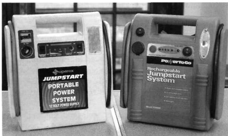
Fig. 12.2 Automotive jumpstart battery packs can supply 12-volt power for telescope accessories. Photo by Paul Hyndman.
