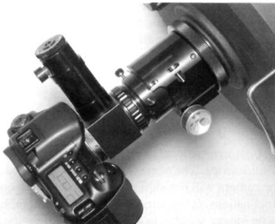
Fig. 9.4 An off-axis guider eliminates differential flexure between the guide scope and the main imaging telescope by allowing the photographer to both photograph and guide on stars from the same telescopic field-of-view. Photo by Robert Reeves.
