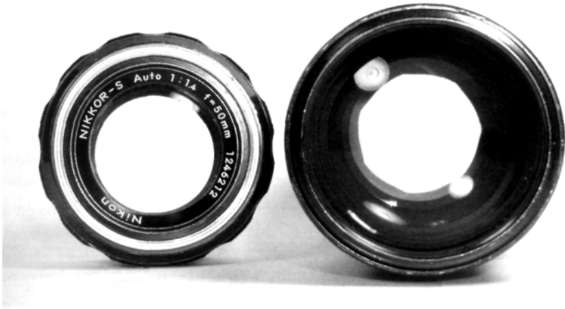
Fig. 7.2 Both the 50-mm f/1.4 and 200-mm f/4 Nikkor set to f/5.6 have a 36-mm aperture and theoretically record stars to the same limiting magnitude. The longer-focus lens will, however, have fewer aberrations, and therefore, sharper focus than the 50-mm lens. Photo by Robert Reeves.
