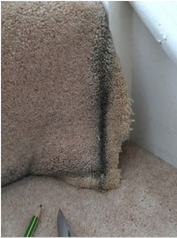
Cutting Taken From Turn - Picture Shows Colour Change Over Time
