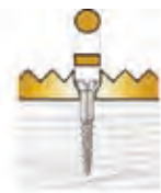
Concealed zinc screw and smooth cover plug (cover plugs should be secured with adhesive)
