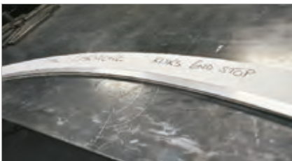
Curved profiles against plan template
