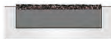
Aluminium Oxide as a surface layer (eg. as in GRP flooring products)
