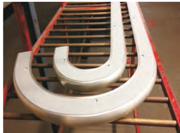
Stair nosing with formed radius end (a 'hockey stick')
