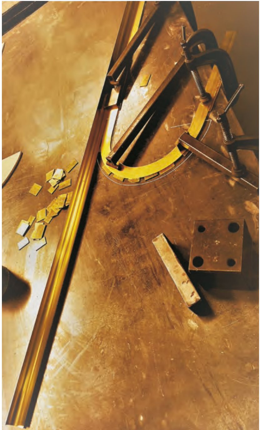
Work In Progress - BN8 stair nosing curving
