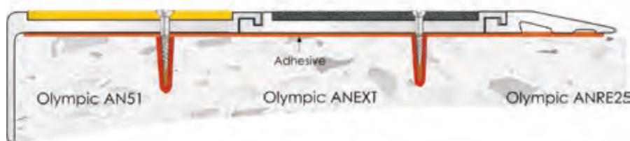
Example of modular combinations and fixing method:
