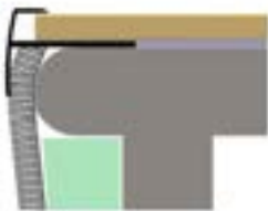
Top Nose fitted with 2mm Underlay and Easyshims to the riser
